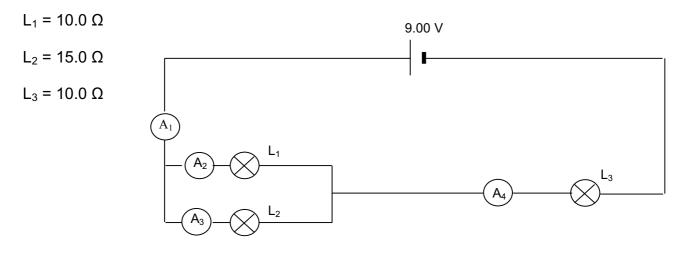
(a) Calculate the total resistance of the circuit.
